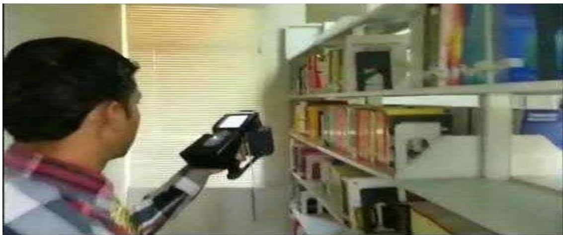
Fig 13: Stock Verification- Moving the RFID handheld reader on the shelf> Note down the Accession Number on the excel sheet
