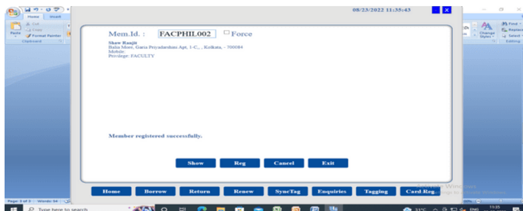
Fig 3: Member Registration- Click on Card Reg option > RFID based smart put on the reader > give the member id (registered on Library Management Software)> press the enter option from PC.
